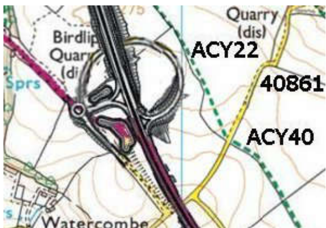
Alternative arrangement with new underpass at the Quarry avoiding diversions of current paths and roads.
